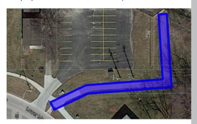
proposed route and then navigate by moving the 'mouse.' If the route will have turning points, the user simply clicks at each turn. Once the route has been completed, the user will click the End Route Button. Clicking the End Route Button will convert the route to an excavation entity with the width previously designated. Clicking on the Edit Locate(s) button allows the user to
